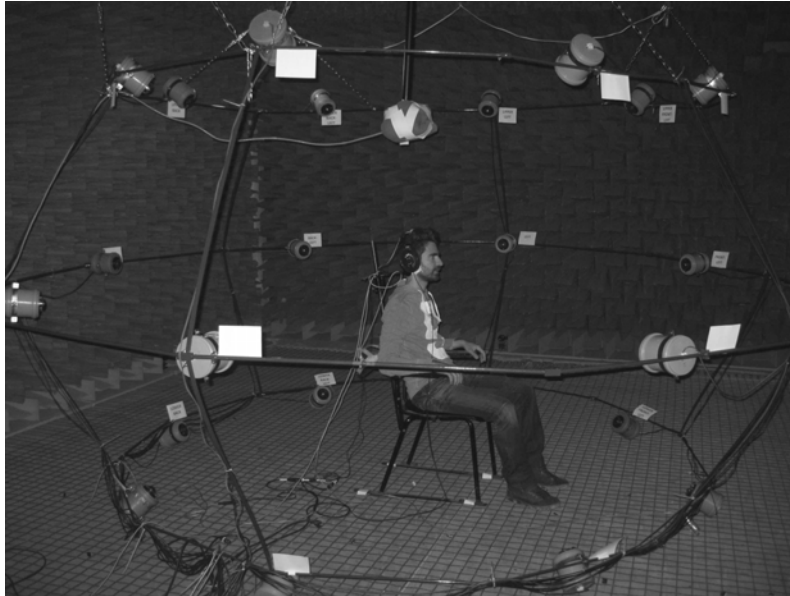
FIGURE 1: Anechoic room with loudspeaker setup and subject.
